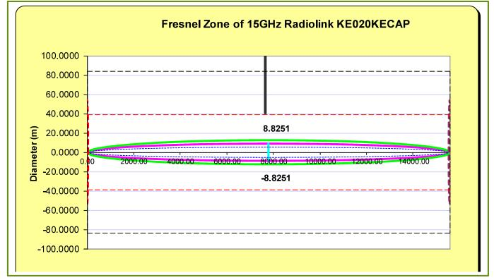
Figure 2 - 1<sup>st</sup> Fresnel zone of Link (1) and proximity of Turbine T10 Rotor Blades
