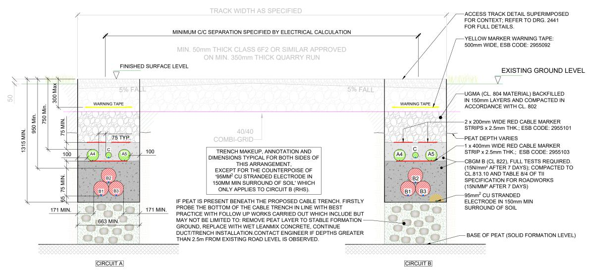
A = 125mm OUTER DIAMETER HDPE ESB APROVED DUCT WITH 12mm DIAMETER PULL ROPES, SDR = 17.6, ESB CODE: 9317553 B = 160mm OUTER DIAMETER HDPE ESB APROVED DUCT WITH 12mm DIAMETER PULL ROPES, SDR = 21, ESB CODE: 9317709 C = 63mm OUTER DIAMETER HDPE ESB APROVED DUCT WITH 12mm DIAMETER PULL ROPES
