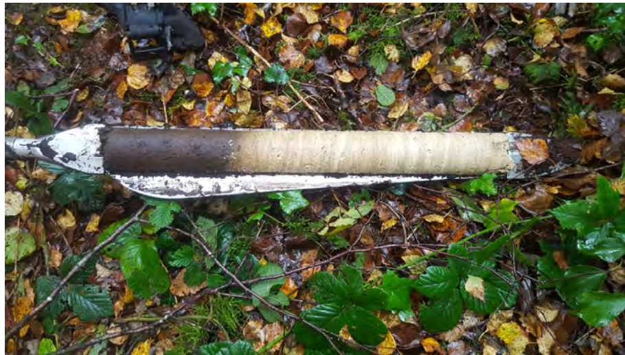
Fig 2.6: Russian core showing soft white shell marl overlain by peat.
